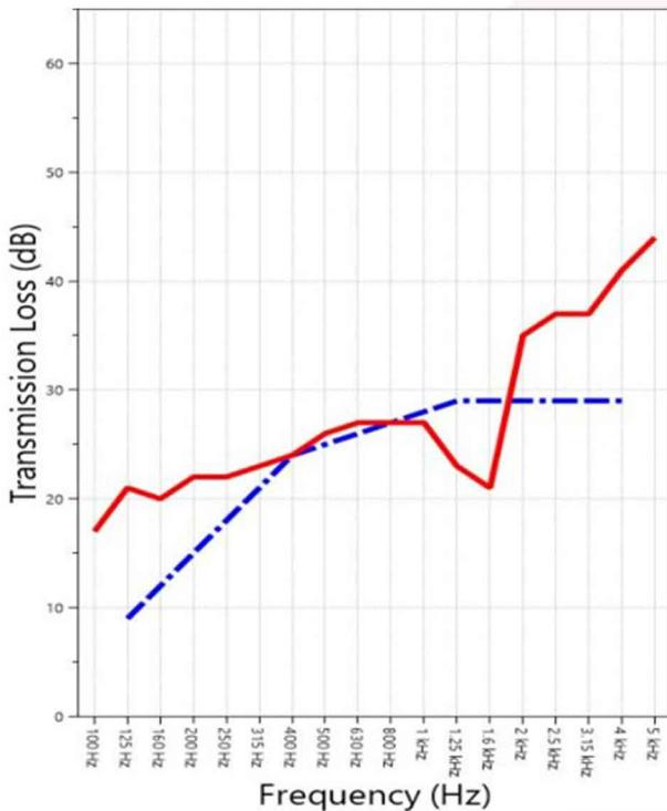
Sound testing was completed at an accredited U.S. Department of Commerce, National Institute of Standards and Technology lab. Across all frequency's tested Barrier Fence sound wall had an average transmission loss of 26 dB. Scoring an STC rating of 25, and an OITC rating of 24.
